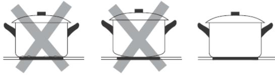
Make sure that the base of the cookware is smooth, sits flat on the hob and is the same size as the cooking area. If smaller diameter cookware is used, efficiency may be lower than expected. Always place the cookware in the centre of the cooking area.
